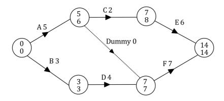
The top number in each vertex is the earliest start time (EST, determined using a forward scan) for the activity that follows, and the bottom number is the latest finish time (LFT, determined using a backward scan) for the preceding activity.
